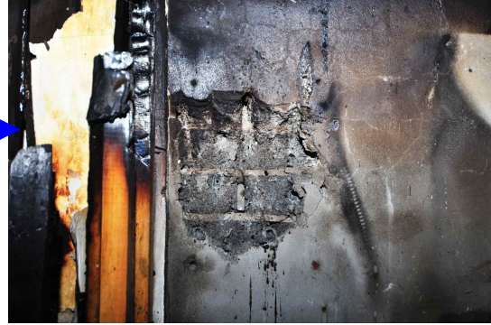
Fig 8. Fire scene of the conductor entrance of the panel board (suspicious ignition point)
