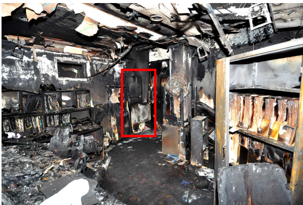
Fig 5. Office on the first floor, panel board combustion
